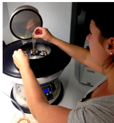
Anna Murphy, wine laboratory manager, loads a sample into the centrifuge for clarifying samples before testing.
